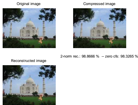
Fig.4 Compression and Decompression of an image using DWT (HAAR Wavelet)
